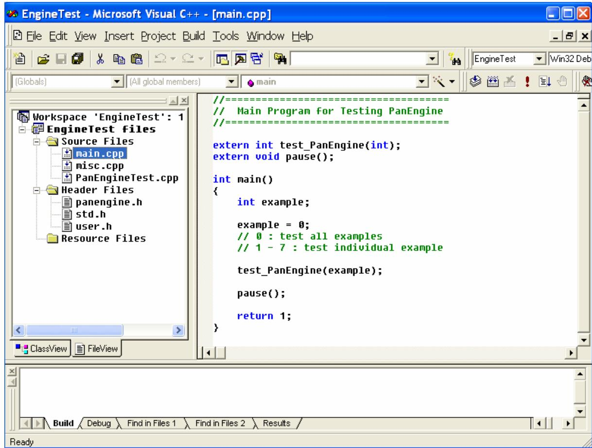
5. Rebuild EngineTest by click **Build** → **Rebuild All**.
