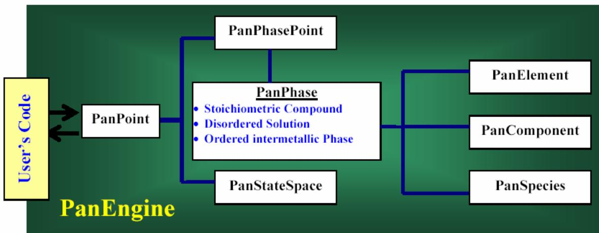
In the CALPHAD approach, the Gibbs energies of all the phases in an alloy system are described by thermodynamic models, such as the ones for stoichiometric phases, the regular-solution-type model for disordered phases, and the sublattice model for ordered phases with a range of homogeneity or an order/disorder transition. These types of models have been implemented in PanEngine.
